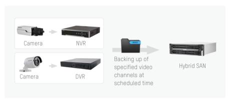
HD video can be stored locally in an NVR or DVR using a LAN. When the network is available, the NVR or DVR transfers video back to Hybrid SAN based on pre-configured rules. This creates an effective video backup solution under restricted data-transmission conditions as, for example, when bandwidth is limited.
